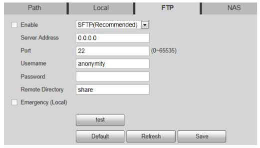
Select **Enable** to enable FTP function, and select the FTP type from the drop-down list.
