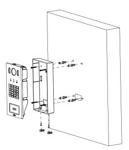
**Step 1** Drill screw holes in the wall according to the position of the screw holes in the mounting box, and then put the expansion tubes in the screw holes.
