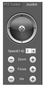
**Notate** PTZ direction through direction button. PTZ supports eight directions: left/right/up/down/upper left/upper right/bottom left/bottom right. Click , and draw a box in the image, PTZ will rotate, focus and quickly position the defined scene.
